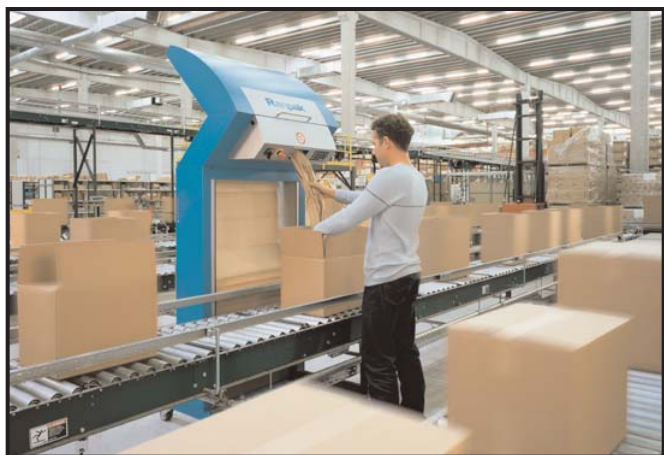
FillPak integration into existing packaging line at a current end user location
